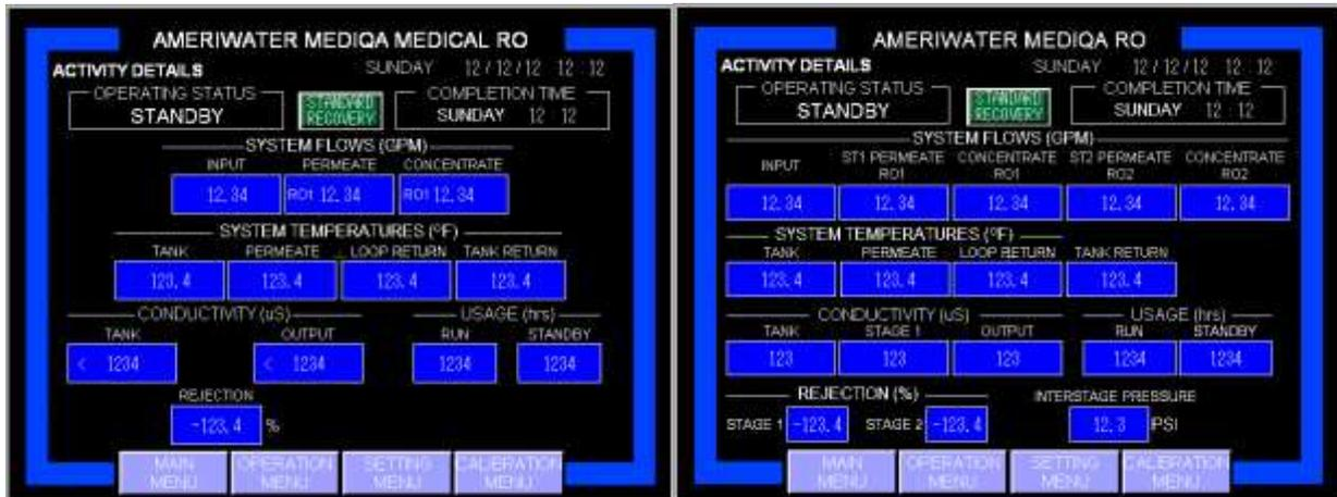
The ACTIVITY DETAILS screen shows specific performance data relating to system processing elements. It also displays the number of hours the MediQA has been running or has been in standby. These can be reset to zero by pressing
