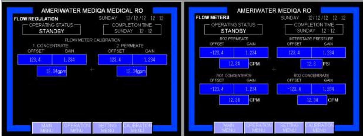
OFFSET and GAIN are calibration parameters. Offset adds or subtracts a constant value to the signal. Gain multiplies the signal by a constant factor.
