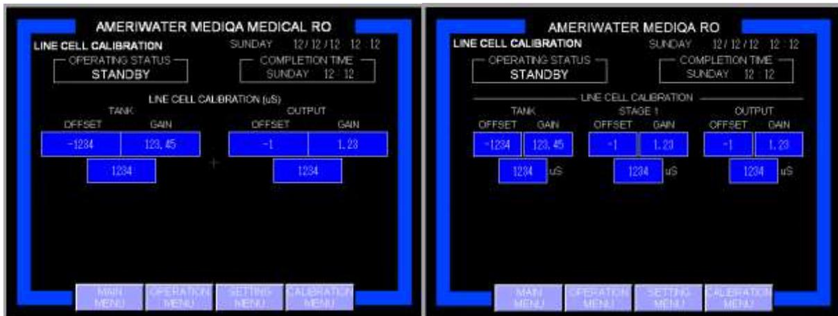
OFFSET and GAIN are calibration parameters. Offset adds or subtracts a constant value to the signal. Gain multiplies the signal by a constant factor.
