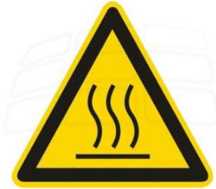
**Hot Surface:** This label is used to indicate that the surface labelled may be hot to touch under certain circumstances during the operation of the unit and in particular during the heat disinfection cycle. Avoid handling any part with this label during heat disinfection or take suitable measures to protect yourself from the heat.
