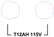
This label identifies the position of the unit's two external fuses. Refer to **Section 12.1.2** for Fuse details and **Section 9.3.11** for replacement instructions.
