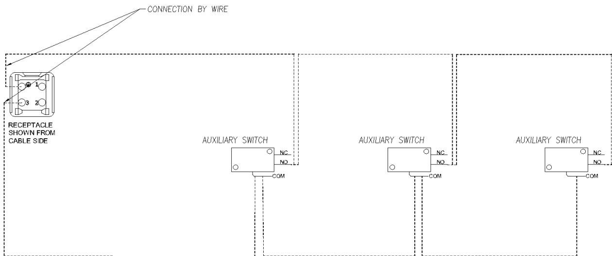
NOTE: THIS DIAGRAM SHOWS THREE VALVES ALL BEING CONNECTED TO THE DELUXE RO WIRING HOOD FOR PRE-TREATMENT LOCKOUT. THIS DIAGRAM IS FOR ALL STANDARD PRO4 RO'S.
