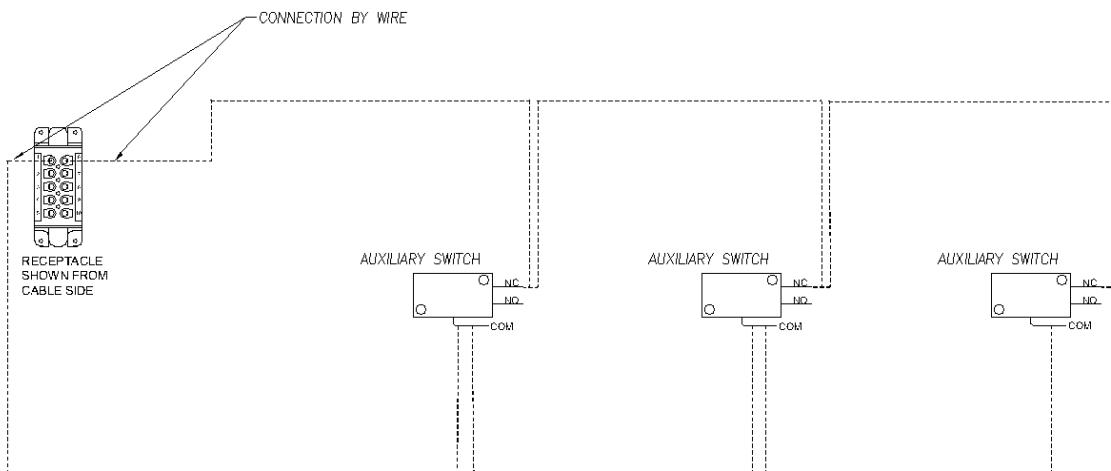
NOTE: THIS DIAGRAM SHOWS THREE VALVES ALL BEING CONNECTED TO THE DELUXE RO WIRING HOOD FOR PRE-TREATMENT LOCKOUT. THIS DIAGRAM IS FOR ALL DELUXE PRO4 RO'S.
