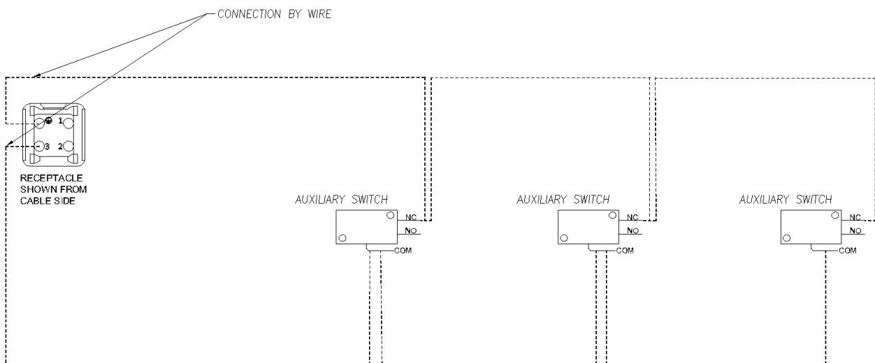
NOTE: THIS DIAGRAM SHOWS THREE VALVES ALL BEING CONNECTED TO THE DELUXE RO WIRING HOOD FOR PRE-TREATMENT LOCKOUT. THIS DIAGRAM IS FOR ALL STANDARD PRO4 RO'S.
