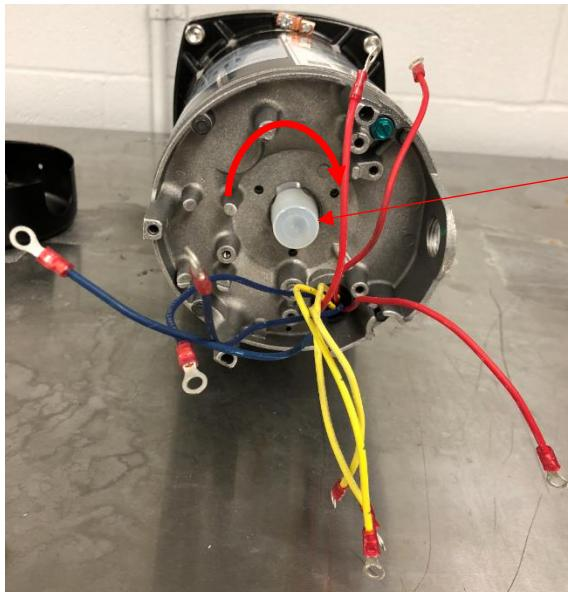
Remove plastic cover to expose motor shaft. Check for correct rotation direction. RO pump shall be labeled with direction of rotation on front of pump.
