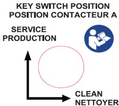
Turn the key switch on the rear of the unit to the **"CLEAN"** position.
