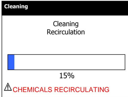
The unit will automatically recirculate the cleaning chemical for approximately 30 minutes and then carry out both high pressure and low pressure flushing cycles so don't be alarmed if the unit sounds different to normal operation.
