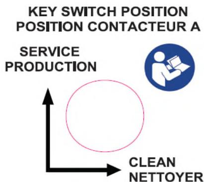
Turn the key switch on the rear of the unit to the “**CLEAN**” position. If this is not selected the unit will revert back to the “**POWER-ON**” screen if a chemical clean is attempted
