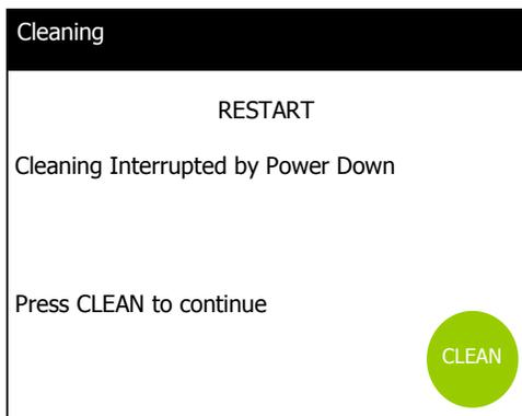
If there is an interruption in the electrical supply the chemical cleaning process will stop. Once the electrical supply is restored a text screen message "**Cleaning Interrupted by Power Down**" will be displayed. Press "CLEAN" to continue. This is to ensure that the unit is fully rinsed free of chemical before further dialysis can take place.
