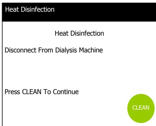
Once the unit's internal tank has filled with the correct amount of water the following message will ask you to disconnect the distribution manifold connection from the Dialysis machine. This will stop any chance of hot water from entering the dialysis machine and possibly causing any damage.
