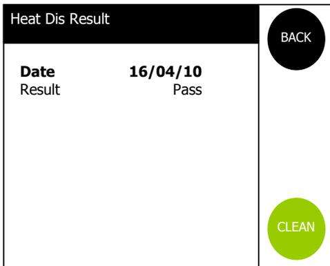
Interrogation of the **Heat Dis Result** screen (from the **Clean** menu) will show the result of the last heat disinfection together with any failure message if relevant. Refer to Section 5 "**Troubleshooting**" and contact your Healthcare provider if necessary
