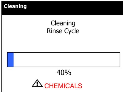
At the end of the recirculation cycle the unit will go immediately into a rinse cycle flushing the cleaning chemicals out of the unit for approximately 45 minutes
