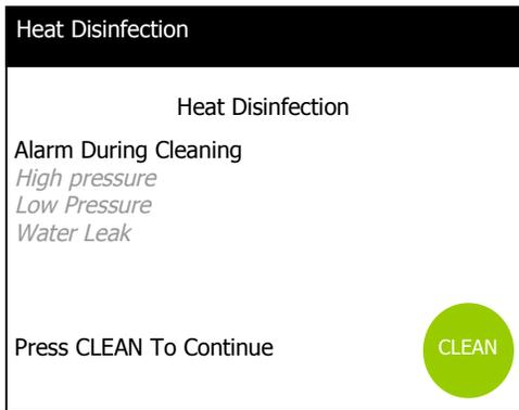
If the unit detects a fault during the heat disinfection process, this alarm screen will be displayed along with a message relating to the possible fault. Pressing 'CLEAN' will resume the process if safe to do so. If pressing "CLEAN" does not resume the disinfection sequence, or the alarm screen keeps appearing, refer to Section 5
