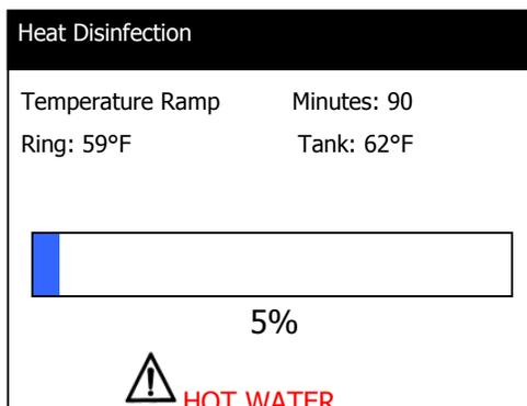
The unit now carries out some internal safety checks. If all checks are complete, the unit will then start to heat the water up. If the unit does not reach temperature within 90 minutes the unit will revert to a rinse cycle and the alarm message "**Heatsan failure**" will be displayed.
